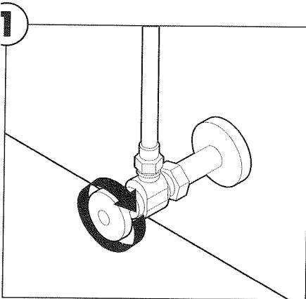
Turn off the water supply, flush the toilet to empty the tank.
