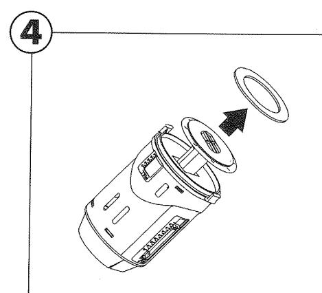
Locate the old seal at the bottom of the canister and peel it off.
