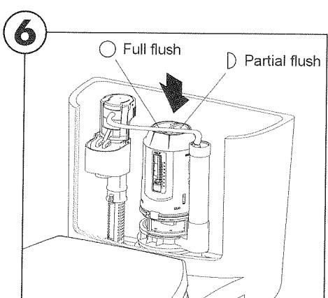
Insert the canister into the base and make minor direction adjustment.
