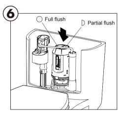
Insert the canister into the base and make minor direction adjustment.
