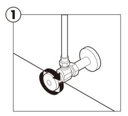
Turn off the water supply, flush the toilet to empty the tank.
