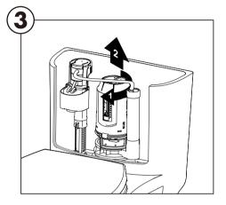
Turn the canister clockwise and lift up to remove.
