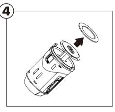
Locate the old seal at the bottom of the canister and peel it off.
